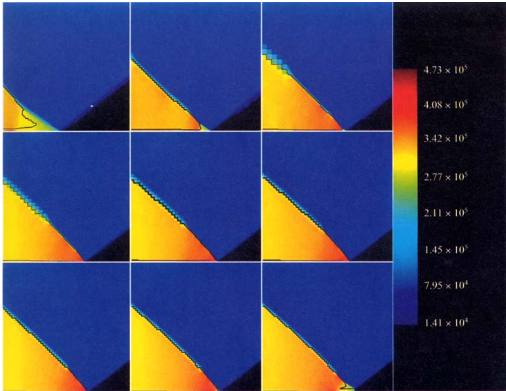
FIGURE 13. Self-similar pressure and self-similar \hat{M} = 1 contour for \gamma = 5/3 , M_i = 2.327 , \theta = 52^\circ . Units are Pa.
